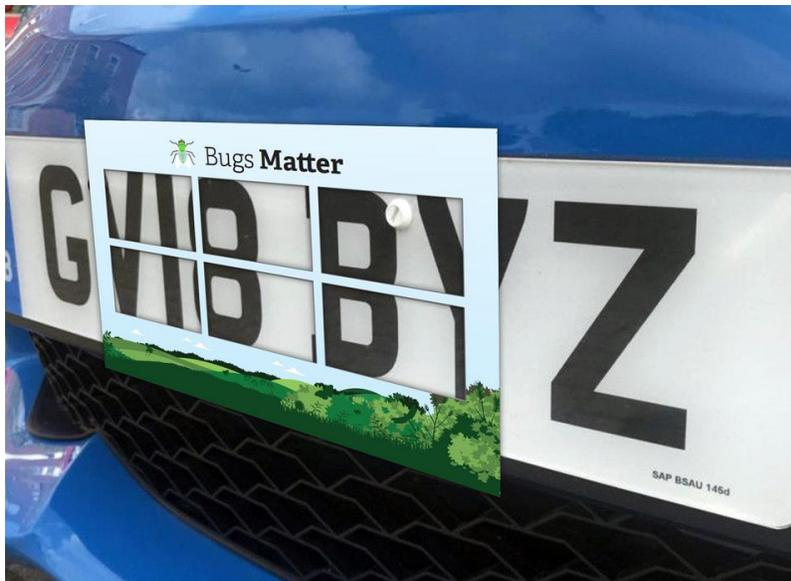
Figure 2. Photograph showing the splatometer positioned over a number plate.
