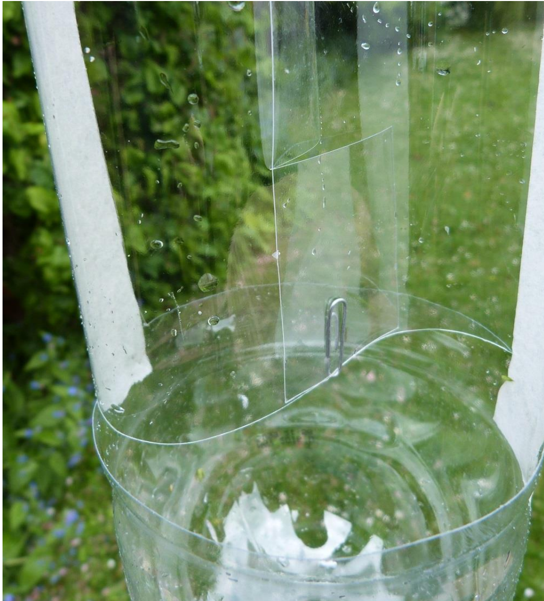
Figure 13: Detail of the aerial interception trap, showing the internal surface of the trap. One aerial bottle trap was deployed at Petworth Deer Park, on a magnificent veteran oak referred to by Denton (2002) and Telfer (2010) as the Barrel Oak, SU962228 (Figure 14, Figure 15).
